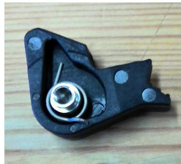
Set up the ensemble on the plate with the cleat in the good way, notice than the cam bothers the spring position, you cannot engage totally the cleat neither the spring. Be patient.Put a tear of a medium screw locker liquid. Engage the screw, at the opposite face of the plate, with the spring loop not engaged. Screw a little bit.
