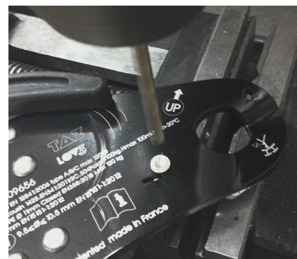
Pay attention to not damage the plate sanding and also drilling, respecting the center of the rivet and drilling only the rivet. Once the hole by drilling is deeper than the head of the rivet, you will drive it out with a hammer and a buffer.
