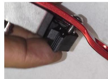
Engage the spring loop in its hole with a tool (thin screw driver or knife arrow) in order to allow the final position of the cleat.
