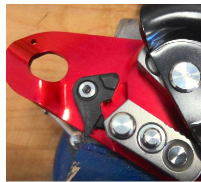
Set up the spring and the axis within the cleat.
