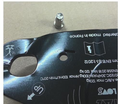
At least, check than the plate hole is not damaged. (In case contact TAZ with photos to assess before reassembly).
